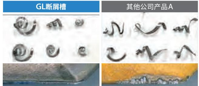
切削参数 :  $V_c = 300 \text{ m/min}$ ,  $a_p = 1.0\text{-}1.5 \text{ mm}$ ,  $f_z = 0.2 \text{ mm/t}$  Q235  $\phi 100$ (15枚刃)
